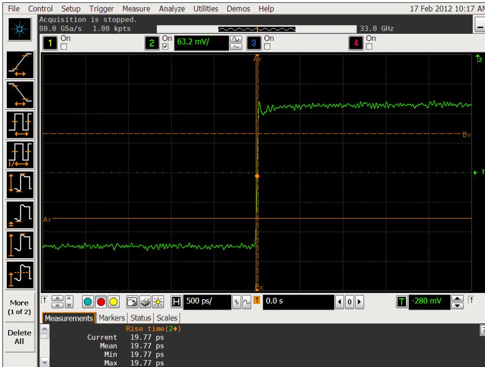
Image 3: Image of the calibration edge of the 90000 Q-Series oscilloscope
