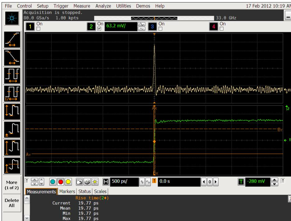
Image 4: Pulse created from differential math of the fast edge
