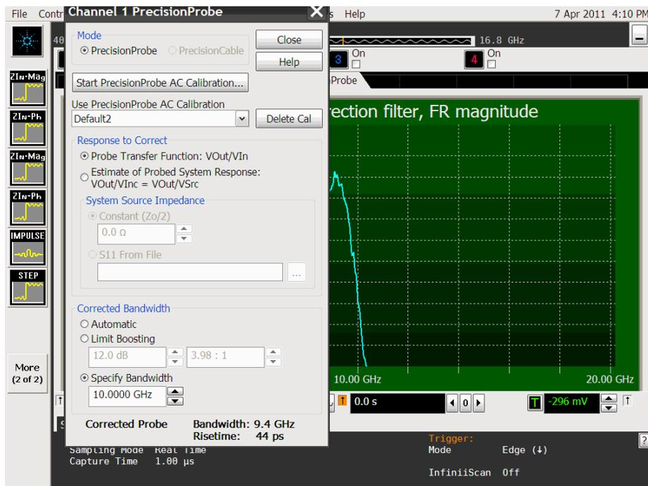
Image 6: Step by step wizard from the PrecisionProbe software
