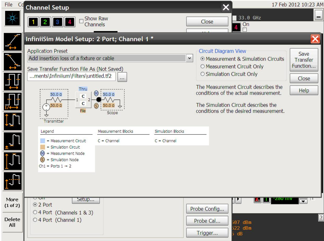
Image 2: Agilent's InfiniiSim software showing how to remove insertion loss through its menu
