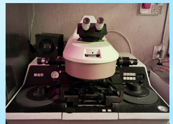
Fig. 2 The Quintel Q2001 mask aligner at the University of Florence.
