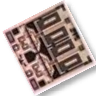
S-band; 20W (CW), 60% PAE, 33dB Gain
