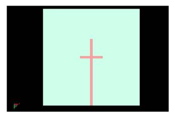
*Figure 3: The microstrip feed line with the impedance matching stub are shown on the bottom of the sub-strate.*
