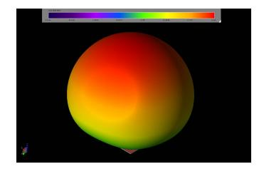
Figure 6: At 1.568 GHz, the gain pattern is nearly spherical and has a peak gain of 5.4 dBi in the direction directly above the dielectric block.
