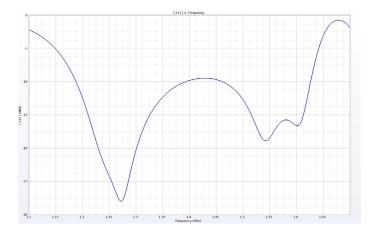
Figure 4: The return loss for the antenna shows two operating bands which correspond to the desired frequencies of 1.268 and 1.561 GHz
