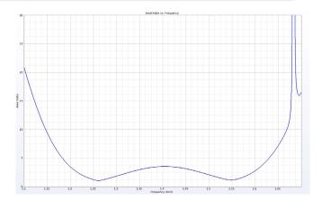
*Figure 8: The axial ratio shows minima near the desired frequencies of 1.268 and 1.561 GHz and fairly broad 3 dB bandwidth.*
