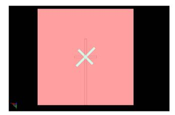
Figure 2: A top view of the antenna structure with the dielectric resonator block removed shows the crossed slots in the ground plane and the outline of the microstrip feed line on the bottom of the substrate.
