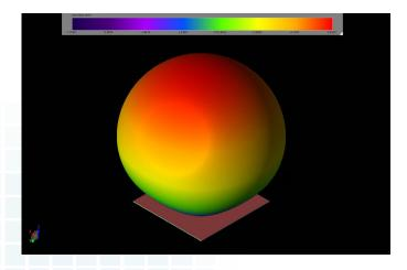
Figure 5: At 1.268 GHz, the gain pattern can be seen to be nearly spherical with a peak gain of 5.6 dBi above the dielectric block.
