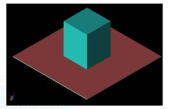
Figure 1: A three-dimensional CAD view of the antenna geometry is shown with the dielectric resonator block visible at the center of the ground plane.
