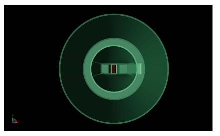
*Figure 3: A view down the horn opening shows the tapered dielectric strip partially filling the center of the high frequency waveguide.*
