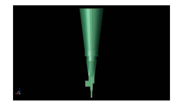
Figure 2: A top view of the antenna shows the orientation of the two input ports and the overall shape of the transition regions and horn.
