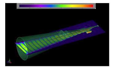
*Figure 6: Time domain electric fields from the 94 GHz port show the propagation through the transition region and out of the horn of the antenna.*
