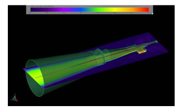
Figure 7: Steady-state electric fields at 94 GHz show field distributions throughout the cross section of the horn.
