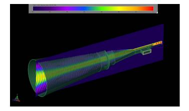
*Figure 8: At 340 GHz, the time domain electric fields are more tightly bound to the tapered dielectric strip in the center of the horn.*
