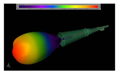
Figure 11: At 340 GHz the gain pattern has a nearly-symmetrical beam with a slightly higher peak gain of nearly 19 dBi. The sidelobes are down nearly 40 dB from the peak.
