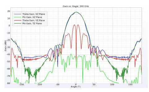
*Figure 13: At 340 GHz, the gain in the principal planes is symmetrical with low side lobes. The cross-polarized fields are higher in one plane but are still down more than 15 dB.*
