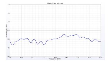
Figure 5: At 340 GHz, the return loss is nearly -20 dB for the high band port.
