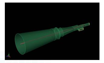
Figure 1: A three-dimensional CAD view of the antenna shows the two input ports to the right and the tapered quartz strip running down the center of the horn structure.
