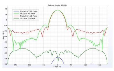
*Figure 12: The gain in the two principal planes at 94 GHz shows a strong, symmetrical beam and very low cross polarized fields.*
