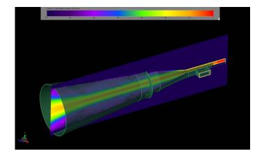
*Figure 9: The steady-state electric field distribution at 340 GHz highlights the stronger fields in the dielectric.*
