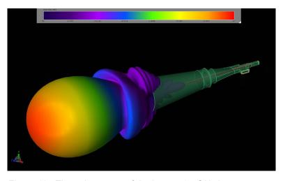
Figure 10: The gain pattern of the horn at 94 GHz has a symmetrical beam with peak gain at 18 dBi and low side lobes.
