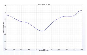
Figure 4: The return loss for the 94 GHz port shows a good match with values below -15 dB.
