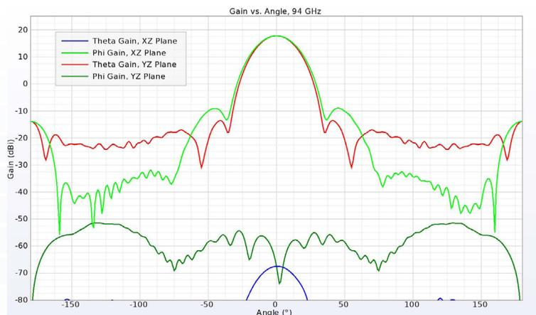
Figure 12: The gain in the two principal planes at 94 GHz shows a strong, symmetrical beam and very low cross polarized fields.
