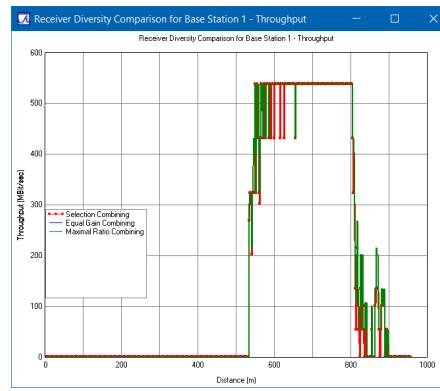
Figure 4: Throughput comparison of receiver diversity methods for base station 1.
