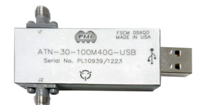
100 MHz to 40 GHz, 30 dB USB Attenuator
