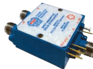
2 to 18 GHz SP2T Absorptive Switch
