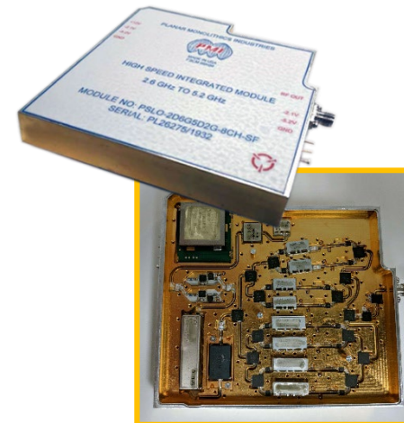
2.6 to 5.2 GHz 8 Channel Selectable LO Frequency Source
