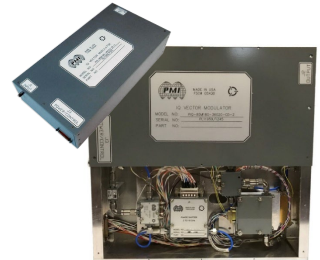
85 MHz to 18 GHz, I/Q Vector Modulator
