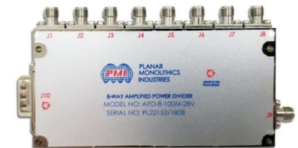
100 MHz, Amplified 8-Way Power Divider
