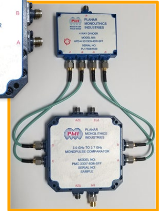
3 to 3.7 GHz Monopulse Comparator
