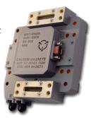
Medium power broadband single pole double throw (SPDT) series of switches are designed for reliable operation at power levels of 5 W, 10 W, 20 W, 50 W and 100 W averages from 100 MHz to 18 GHz. These are robust PIN diode switches with proven field reliability. Proprietary PIN diode architecture minimizes junction temperatures to assure long life under medium power conditions.
