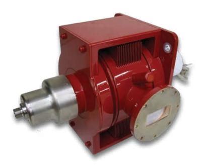
A magnetron is a high power microwave oscillator in which the potential energy of an electron cloud near the cathode is converted into RF energy in a series of cavity resonators. The VMC3109 magnetron delivers high peak and average RF power for use in medical or industrial applications.
