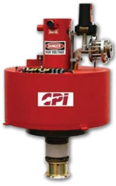
The VKX-8253A is an electromagnet focused, 9.3 GHz klystron which has demonstrated peak power of 5.5 MW with 18 kW average, at an RF pulse width of 9 µs. The klystron achieved power of 6 MW peak at 6 kW average. The unit was designed to achieve 20 kW average power at 5 MW peak
