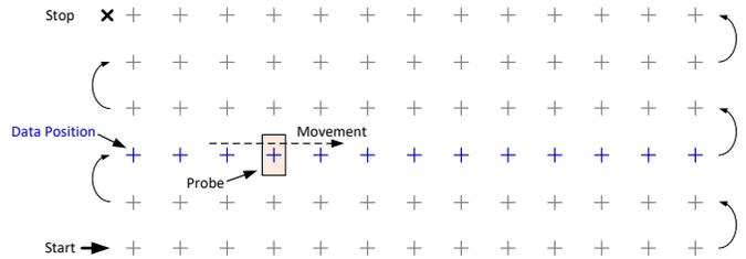
The motion controller is configured to produce a Trigger pulse *before* each point is reached, so that a complete set of measurements will be centered on the desired position. Because the direction of movement is reversed, the trigger positions differ between forward and reverse lines.
