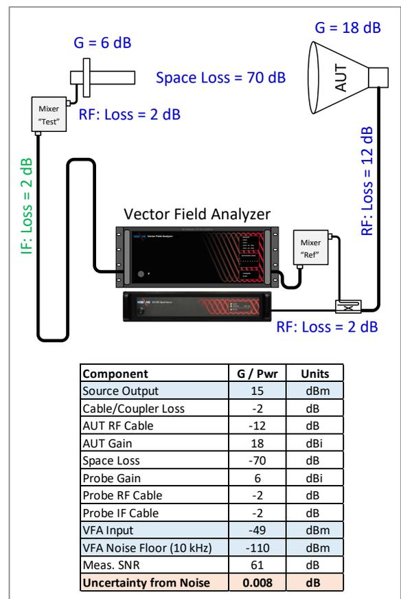
us to eliminate almost all the probe cable's loss. The compact remote mixer mounts at the probe, and converts the test frequency down to a much lower intermediate frequency (IF) where cable loss is greatly reduced. The VFA is designed around remote mixers, and offers this advantage in multiple, broad frequency ranges. It can also be configured with internal mixers for simpler, smaller measurement tasks where cable lengths are not so critical.
