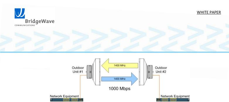
Figure 7 - 80 GHz Gigabit Configuration
