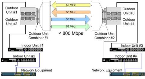
Figure 4 - Dual RF Channel Configuration, Implementation "A"
