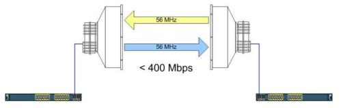
Figure 3 - Single RF Channel Configuration, All-Outdoor
