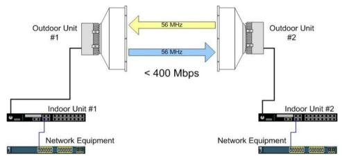
Figure 2 - Single RF Channel Configuration, Split Mount
