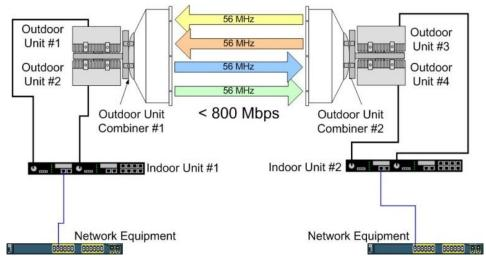
Figure 5 - Dual RF Channel Configuration, Implementation "B"
