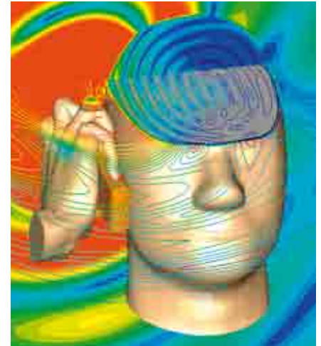
EM field distribution of a Sony Ericsson mobile phone at 1.8 GHz for SAR analysis: the mobile phone's CAD data was imported using the STEP interface and combined with a hand and SAM model.
