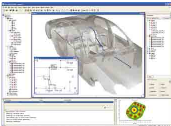
Position and cross-section of a cable harness inside a car: surface currents can be used for EMC analysis.
