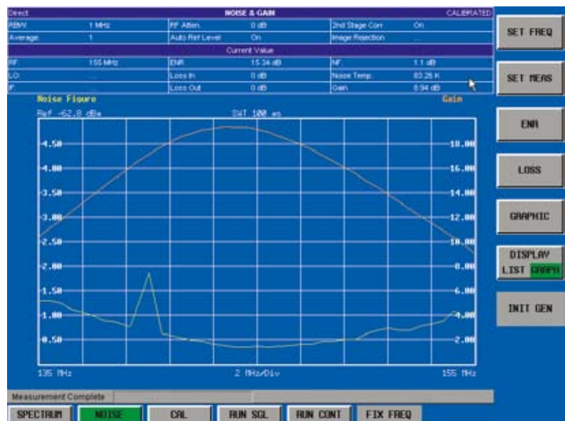
Measurements on a GaAs preamplifier show an anomaly at 140 MHz; its cause can easily be traced in the spectrum analyzer mode
