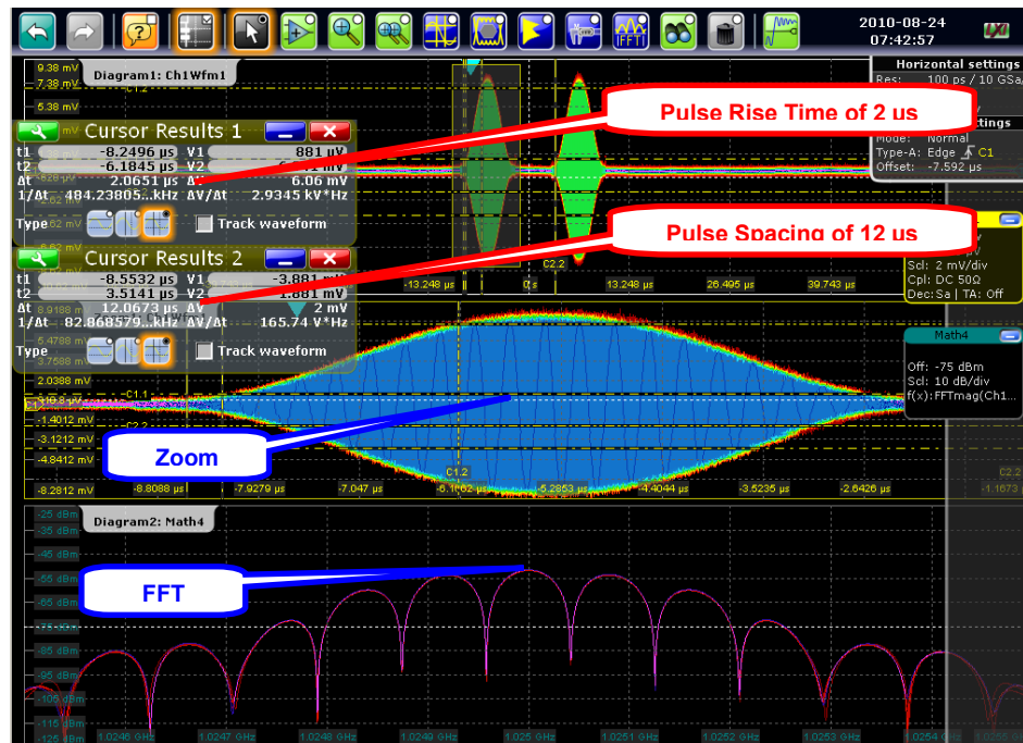
Figure 45: R&S®RTO digital oscilloscope with DME pulse analysis and FFT spectrum.
