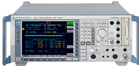
Figure 24: The R&S®FS-K15 avionics option for VOR/ILS transmitter testing installed in the R&S®FSMR measuring receiver.
