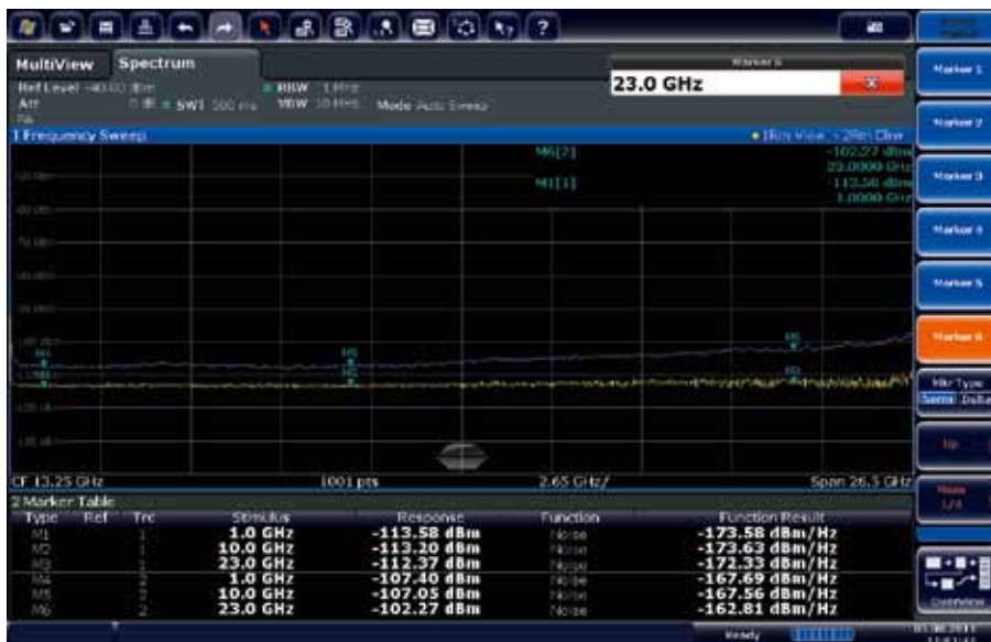
Displayed average noise level (DANL) with preamplifier and noise cancellation switched on.
