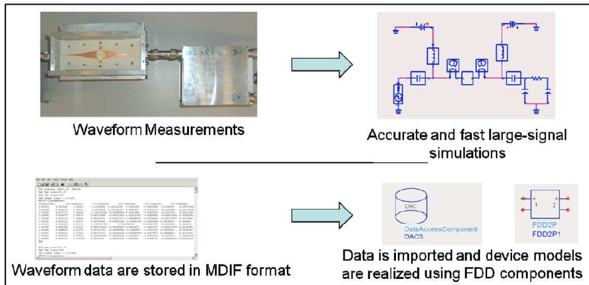
Figure 5. Workflow for exporting waveforms to EDA software tools.
