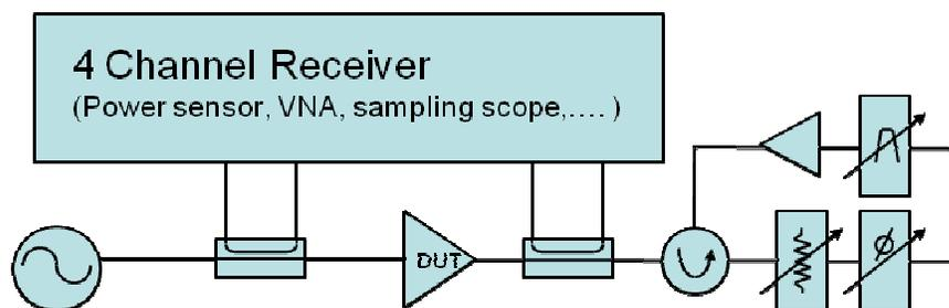
Figure 2. Closed loop, active load pull test set up
