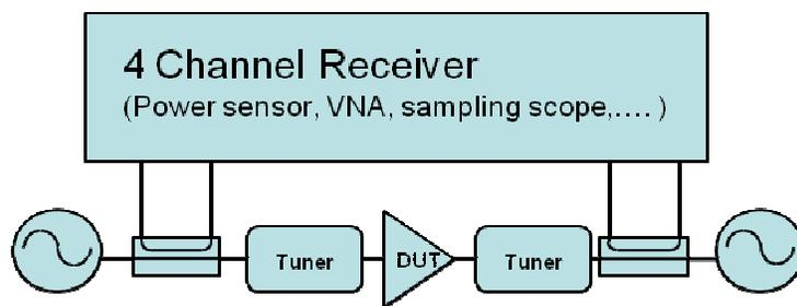
Figure 1. Passive source, load pull test set up.
