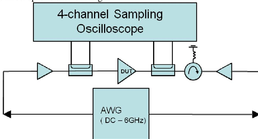
Figure 4. Test configuration for open loop, active source/load pull.
