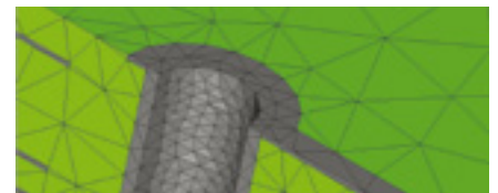
Fields and surface currents of a via, mesh view of PBA, and tetrahedral discretization.
