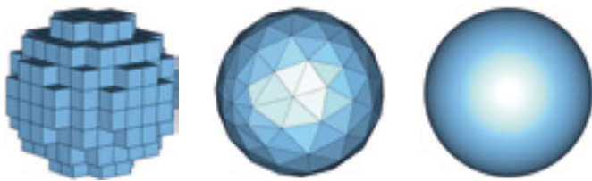
Various meshing strategies for a simple sphere: staircase, tetrahedral, and CST's proprietary technology PBA.
