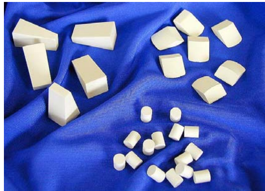
Figure 3. ECCOSTOCK® HiK is a low-loss dielectric material. The smallest slugs/barrels, pictured here, were used in a phased-array antenna for Boeing's Connexion program.
