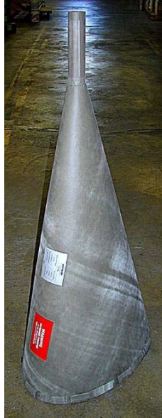
Figure 2. This ECCOSORB® ANW-73/ML removable absorbent cover was constructed to fit tightly over an aircraft nosecone for ground-based radar testing. It acts as a radiation shield that can be easily slid on and off the nosecone during testing. The “W” stands for weatherproofing and refers to the covers inclusion of a neoprene based fabric material which meets MIL-PRF-26096F and is resistant to fuels, lubricants and hydraulic fluids.
