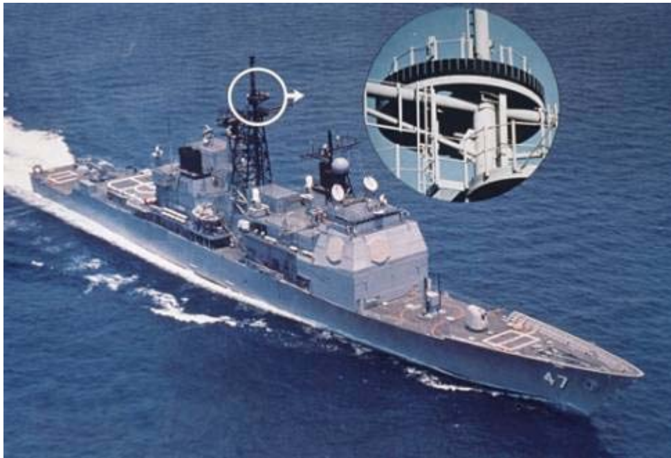
Figure 1. The AIMS antenna group, used shipboard, is comprised of an antenna, antenna position programmer and a below-deck control unit used to locate and identify aircraft as friend or foe. The AIMS antenna consists of 64 radiating elements arrayed in a circle (at right in black) and uses the ECCOSTOCK® SH dielectric material around the ship's mast. Unlike conventional IFF systems, which employ mechanically rotated antennas, the AIMS antenna elements remain stationary while the beam is steered electronically to scan a full 360 degrees around the ship. The beam can also be positioned selectively in any direction within microseconds and has a continuous scan rate of up to 90 revolutions per minute. AIMS is used on U.S. Navy CG 47 class cruisers, DDG 51 class destroyers, LHD 1 class helicopter assault ships, LPD 17 landing platform docks, and the CVN 68 class aircraft carriers.
