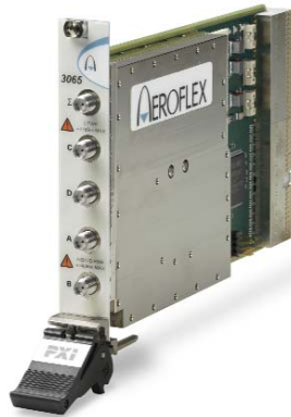
Single slot combination RF switch and power combiner module
