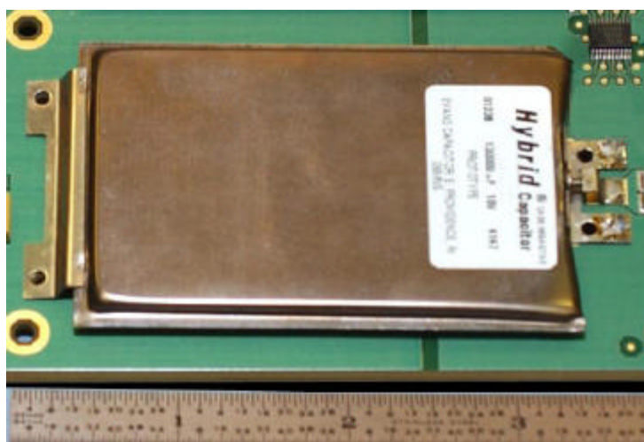
Figure 2. Photograph of the capacitor. The connections are made by soldering directly to the terminals as shown at the right center of the figure. The overall dimensions are 3.07" X 1.98" X 0.21". This device weighs 105g.
