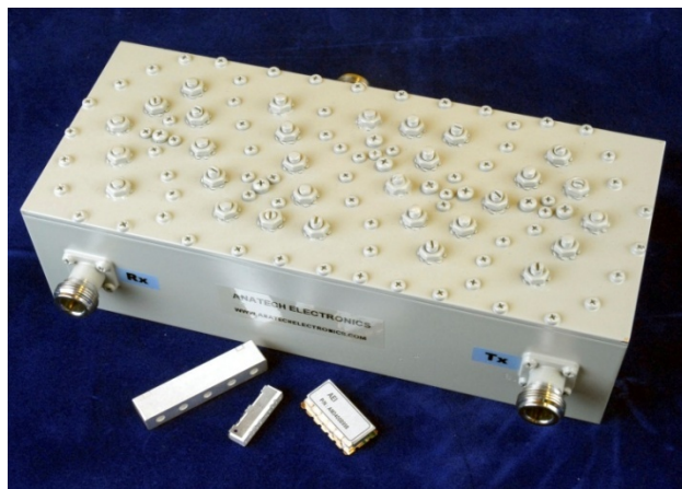
Figure 5 – Size comparison between cavity and ceramic filters
