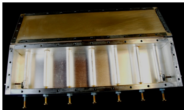
Figure 4 – Inside a cavity filter
