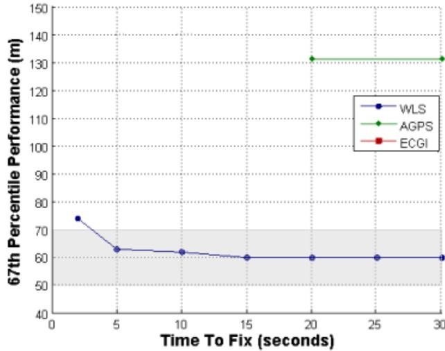
**Figure 3. Polaris WLS accuracy and time to fix compared against A-GPS for all indoor fixes.**
