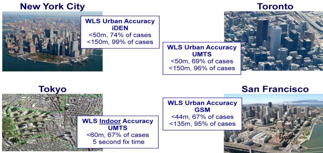
**Figure 2. Polaris WLS accuracy for different cities on iDEN, GSM and UMTS for outdoor and indoor use cases.**
