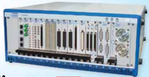
40-923A 19-Slot PXI Modular Chassis
