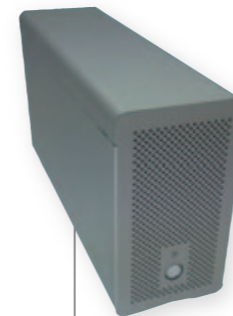
External 3 slot PCIe docking station. Small expansion box for a standard PC (PCI Express) or a Laptop (Thunderbolt)
