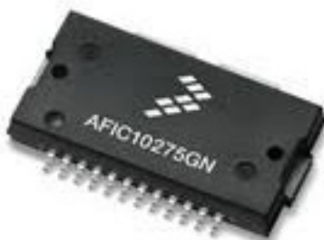
Figure 6: NXP AFIC10275GMR1 two-stage LDMOS amplifier IC
