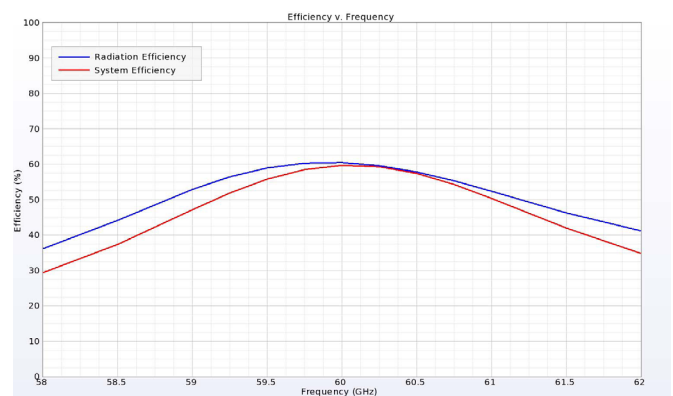
Figure 6: The radiation and system efficiencies of the antenna are quite good at around 60% at 60 GHz due to the reduced losses compared to metal antennas.
