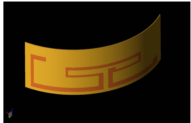
Figure 2: One of the two identical multiband antennas in the remote camera.
