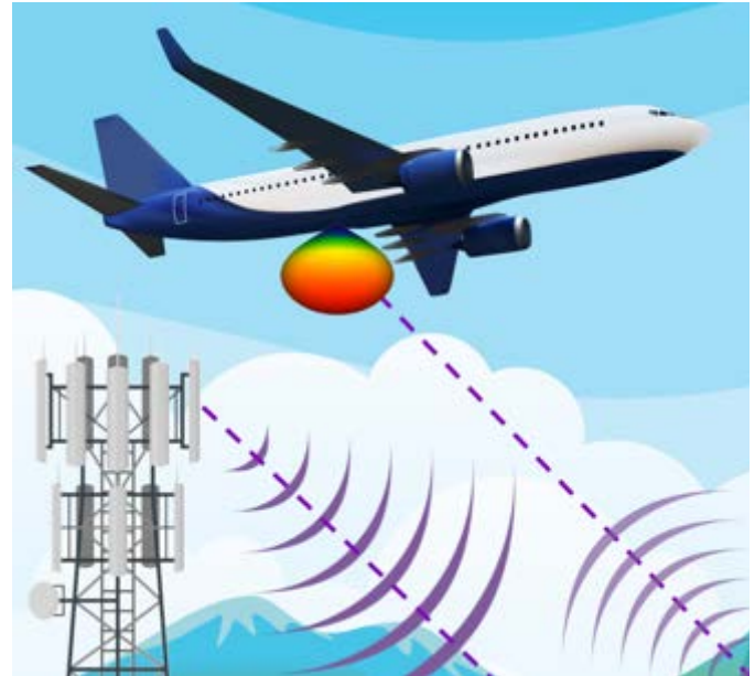
Figure 2. Depiction of 5G radar altimeter interference scenario.
