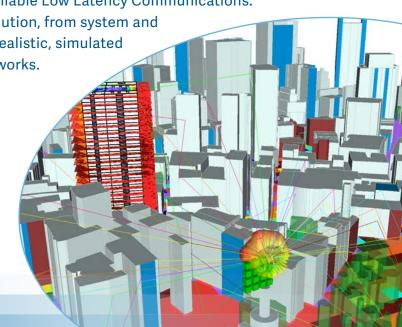
Remcom's unique ray tracing tools simulate MIMO antennas for 5G, WiFi, and other applications relevant to today's rapidly advancing technologies:
