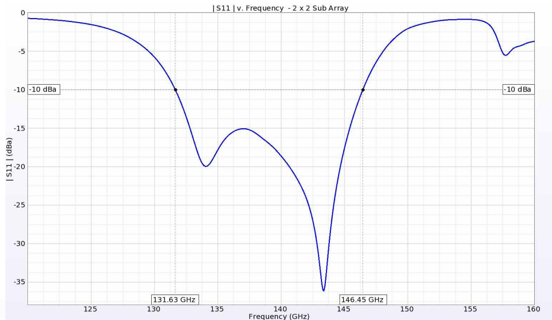
Figure 5: The return loss for a single 2x2 antenna element shows good performance below -10 dB from about 132 GHz to 146 GHz.
