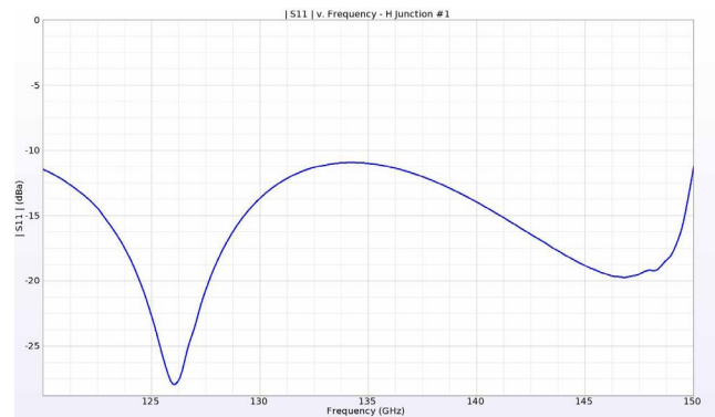
Figure 12: The return loss for the primary H-junction has good performance over the entire frequency range of interest.
