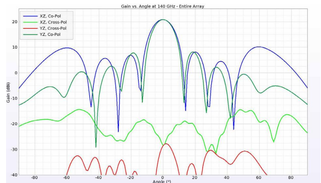
Figure 22: At 140 GHz the sidelobes get slightly larger but remain at least 10 dB down from the peak.
