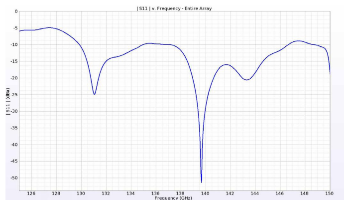
Figure 18: The return loss for the entire array is mostly below -10 dB from 130 to 146 GHz.
