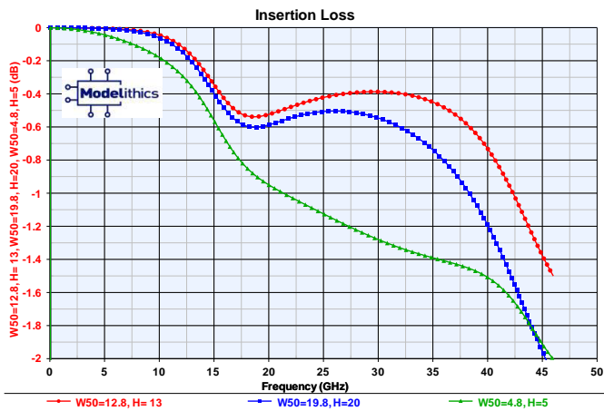
Fig. 12 Insertion loss, 0201BB104 three K=9.6 (alumina) substrate thicknesses, three 50-Ω linewidths
