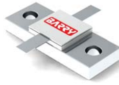
Rated Power: 250W Substrate: AlN Flange: Ni Plated Cu Footprint: 0.975" x 0.375"
