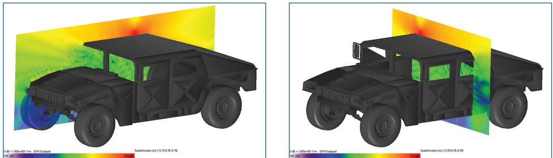
Figure 5: Assessment of fields and potential radiation hazard to driver and passengers using XFDTD
