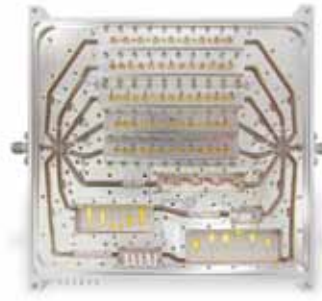
Switched Filter Bank
