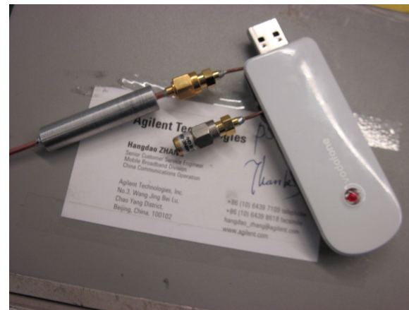
Modified dongle with balun on cables
