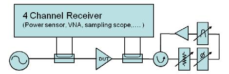
Figure 2. Closed loop, active load pull test set up
