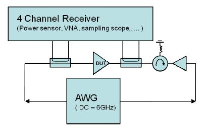
Figure 3. Open loop, active load pull test configuration
