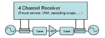
Figure 1. Passive source, load pull test set up.
