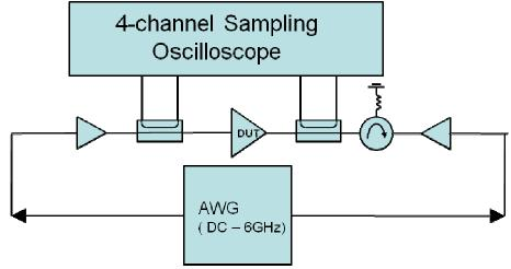
Figure 4. Test configuration for open loop, active source/load pull.
