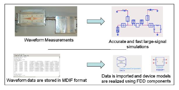
Figure 5. Workflow for exporting waveforms to EDA software tools.
