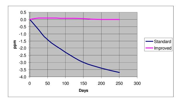
Figure 3: Aging at 85°C. Comparing a typical SMD crystal's aging to the improved TCXO's used for the OCXO equivalent (Pletronics OeXO<sup>TM</sup> Series).
