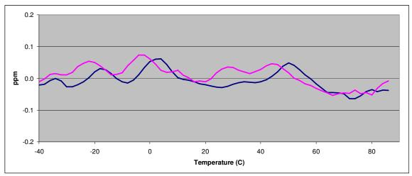
Pletronics OeD4 device operated -0° C to 85° C. Showing hot-to-cold and cold-to-hot temperature changes.
