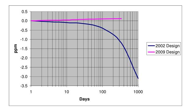
Figure 2: Aging at 77° C. Improvements in performance of the SMD crystal design and fabrication.
