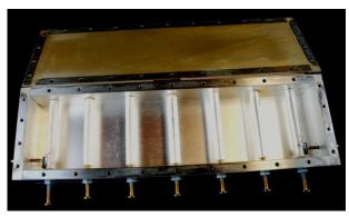
Figure 4 - Inside a cavity filter
