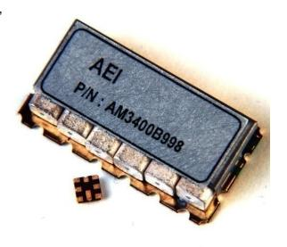
Figure 7 – SAW filter compared to ceramic filter
