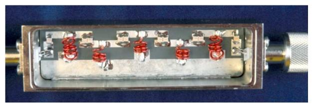
Figure 1 - A typical LC filter
