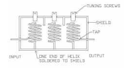
Figure - 10 Helical filter structure
